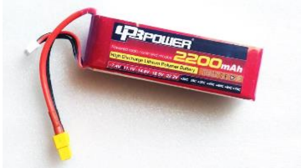
Gambar 5. Baterai LiPo 2200 mAh (Sumber : Hidayat, 2018)
