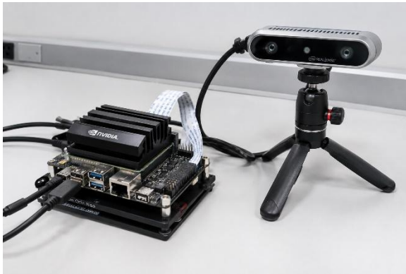
Figure 3. Hardware-in-the-Loop (HIL) testbed for Edge AI processing, featuring the NVIDIA Jetson Orin Nano module paired with a stereo depth camera for local Visual Odometry execution.
