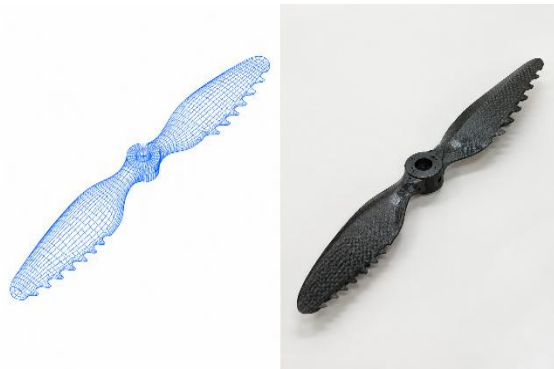
Figure 1. Computer-Aided Design (CAD) wireframe model of the bioinspired trailing-edge serrations (left) alongside the physical FDM 3D-printed PETG-CF rotor prototype (right).
