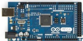
Gambar 2. Arduino Mega 2560
